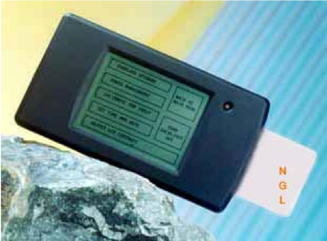
SmarTTouch terminal by NanoGlobes Ltd, is a hand-held smart card data transaction terminal which utilises the latest Liquid Crystal touch screen display technology. Commands and required actions are selected from the on-screen menu by simply touching the LCD with a stylus or a pen. The LCD has a large 320 x 240 dots capability and has a viewing area of 80mm x 62mm.
